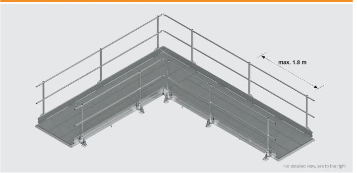
The escape route system from INNOTECH, using concrete slabs, is held in place by its own weight and installed without roof penetration.
