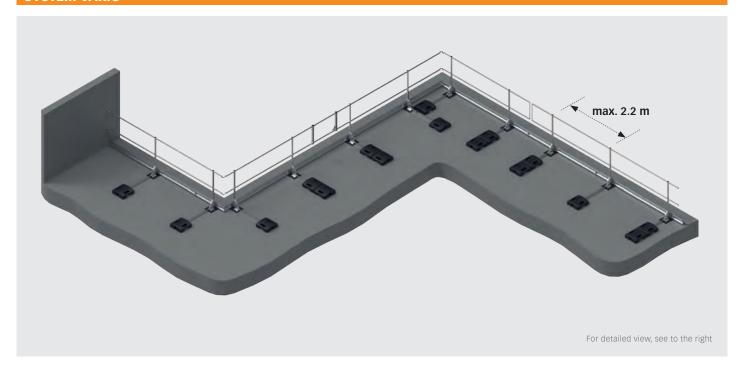
The self-supporting BARRIER VARIO guardrail system by INNOTECH can also be quickly installed retroactively. The system can be adjusted in height by 125 mm, so it adapts ideally to any roof slope. If needed, the railing can be inclined or folded by up to 75°, so the system fits outstandingly into the constructional circumstances.
