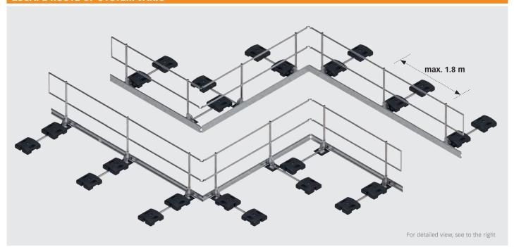
The SYSTEM-VARIO escape route from INNOTECH is self-supporting and thus installed without roof penetration. The width of the flexible system is adjustable, requires significantly less material due to the large distances and thus reduces the superimposed load.
