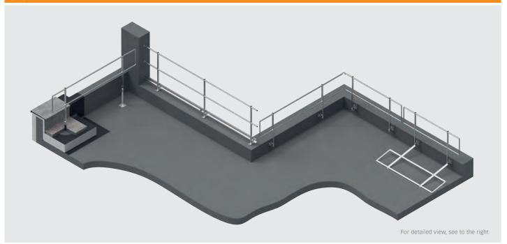
Another solution of the BARRIER guardrail system from INNOTECH consists of installing it on the parapet as the substructure. The guardrail system can be fastened either onto the parapet or to the inside of the parapet. The inclination of the system can be easily adjusted (90°, 70°). In order to maintain the aesthetics of the building, it is possible to fold the system completely.
