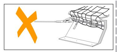
AS FALL-THROUGH PROTECTION SYSTEM IN ACCORDANCE WITH EN 1263-1 AND ANCHORAGE DEVICE ACCORDING TO EN 795:2012 TYP B
