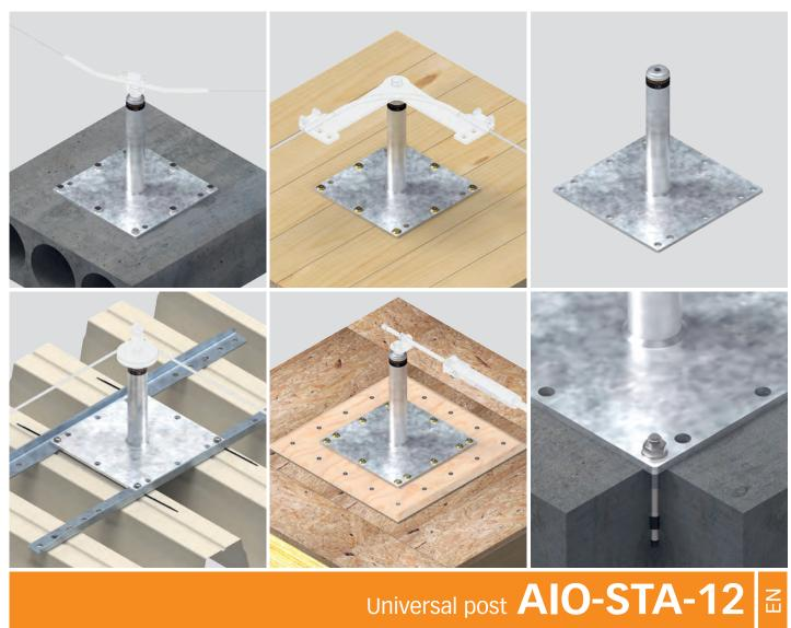
The AIO-STA-12 universal post from INNOTECH can be used as a single anchor point and a system post in the AIO lifeline system. A wide range of fastening sets ensure that it can be installed on almost all substructures.
