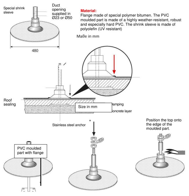
Heat the shrink sleeve collar from the bottom to the top
